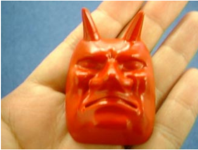
Figure 11: Demon model made by CAM system.
