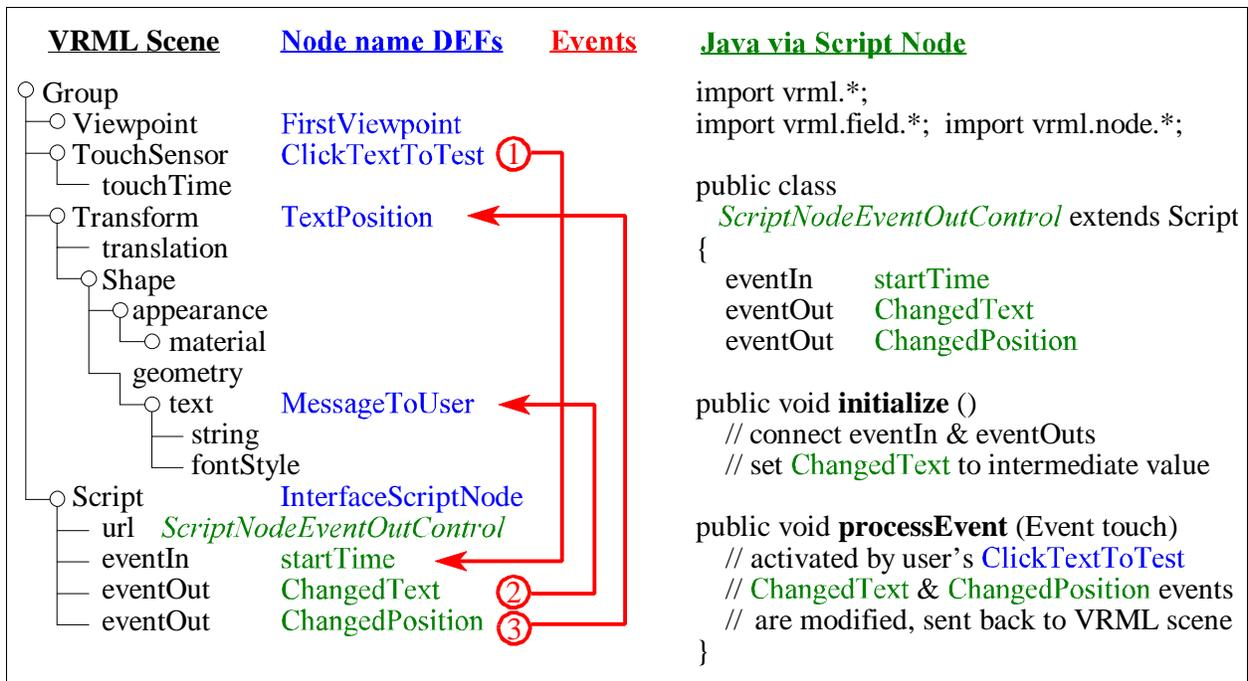
**Figure 4.** Script node interface between VRML and Java. This example tests event-based VRML-Java functionality. Note shared events *startTime*, *ChangedText* and *ChangedPosition*. The following sequence of events occurs:
