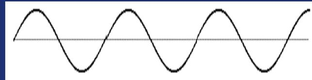
$$\text{Frequency} = \text{Speed of sound} / \text{Wavelength}$$
