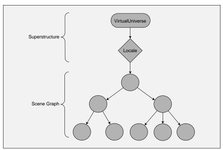
*Figure 7: Java 3D scene-graph nodes are rooted to a* Locale *object that is in turn rooted to a* VirtualUniverse *object.*
