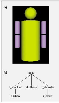
Figure 3: (a) VRML humanoid; (b) Corresponding scene-graph diagram based on human.wrl.
