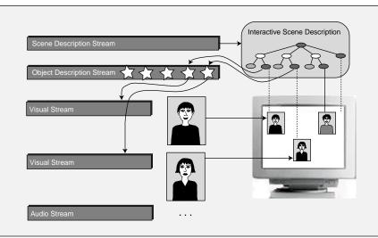
*Figure 5:* MPEG-4 media streams are composed at the terminal according to a scene description.
