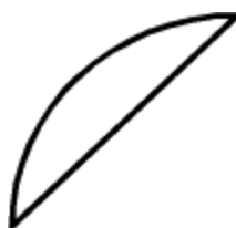
Figure 14.3 — ArcClose2D node ("CHORD" closure)
