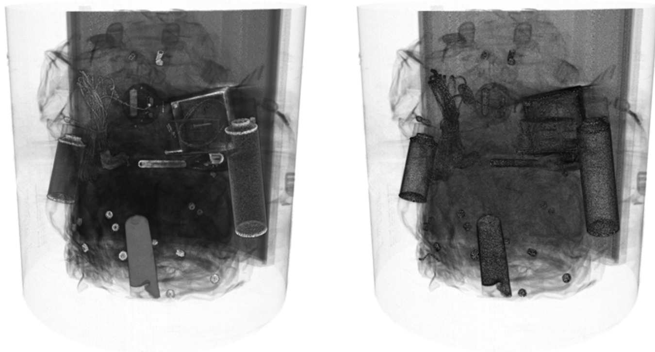
Figure 41.3 — Default volume style on left and CartoonVolumeStyle on right
