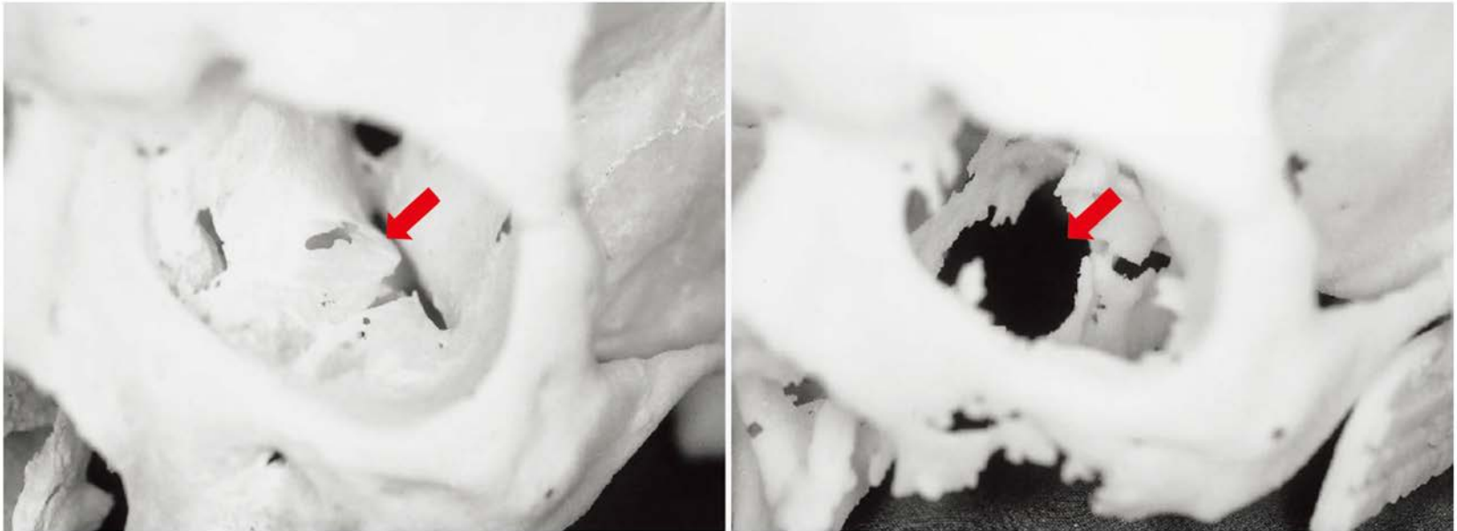
Figure 2. Photographs of a cadaveric skull (left) and the corresponding 3D printed model (right) show a loss of detail in the orbital floors (arrows) and along the margins of a maxillary defect, where the bone is thin, on the 3D model.
