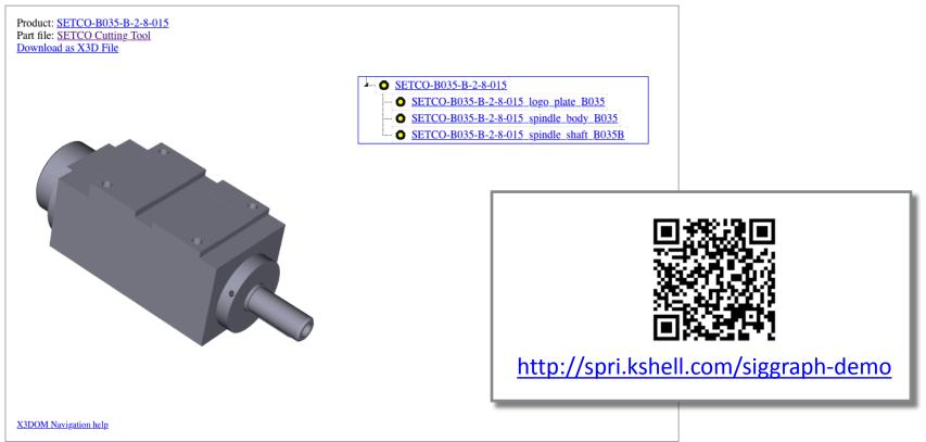
This webpage displays an X3DOM model generated by direct conversion of a STEP (ISO 10303) file uploaded to a web application at <u>http://spri.kshell.com</u>. The assembly structure defined in the STEP file was automatically mapped into the part-assembly nodes defined in the X3D CADGeometry component, and is used to generate a Javascript-based assembly structure viewer on the page.
