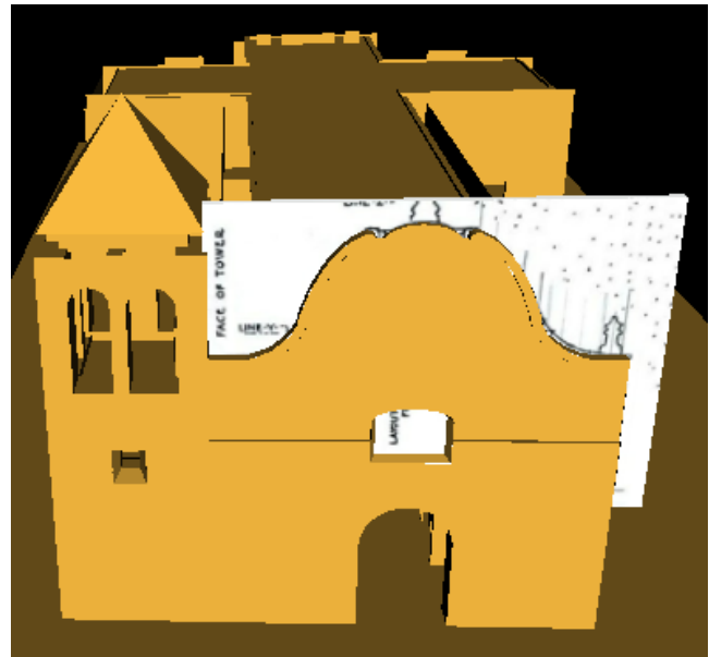
Figure 10: A trick to create curved shapes with the IndexedFaceSet X3D node: a section is attached on a box as a texture, the box is positioned above the façade, the IndexedFaceSet arc is shorten and stretched till it is superimposed on the corresponding arc on the section image.
